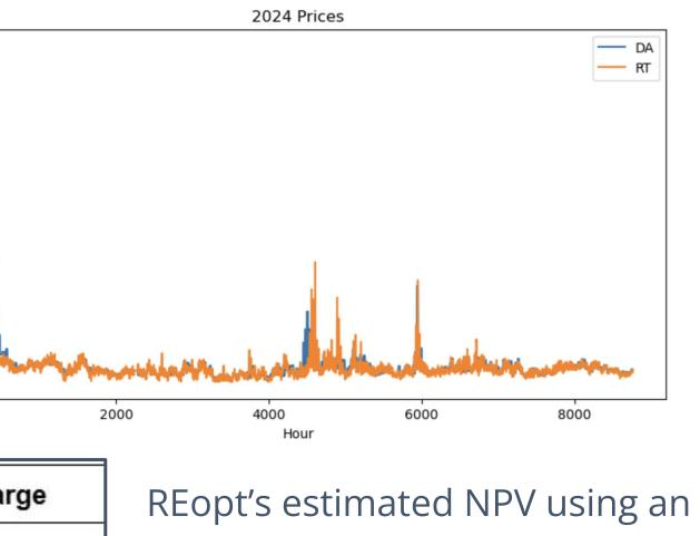
8 MW battery over a 10 year lifetime, based on 2023's DA and RT market data and electrical load, while varying battery usage and applications
